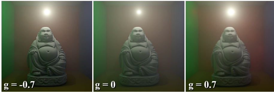
Figure 6.8: The Buddha in a homogeneous medium ( \sigma_s = 0.075 , \sigma_a = 0.001 ) with anisotropy parameter g of the Henyey-Greenstein phase function varying from backward, to isotropic, to forward scattering. Image taken from [46].
