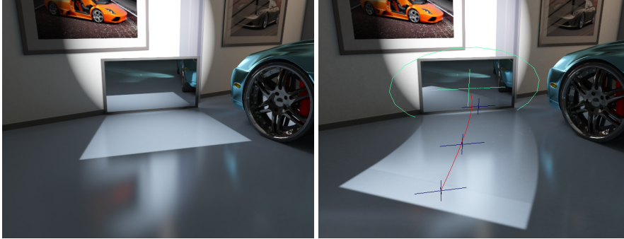
Figure 9.5: Bending paths to form “BendyCaustics” off the mirror. Image taken from [200].
