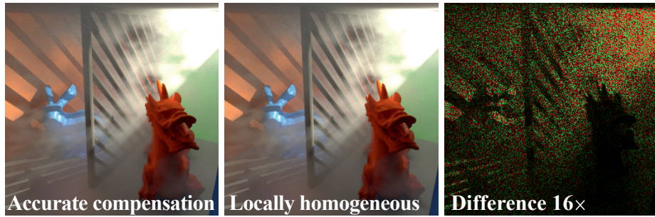
Figure 6.3: Bias compensation with accurate transmittance and with locally homogeneous assumption. Image taken from [46].
