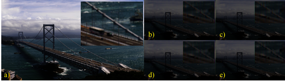
Figure 4.11: Different (subpixel) filters employed in the user study (RGB stripe layout). a) Reference image. b) Mitchell filter, no subpixel rendering. c) Box filter, subpixel rendering. d) Mitchell filter, subpixel rendering. e) Our optimal filter, subpixel rendering. Filtered images are dimmer due to simulating subpixels with real pixels. Although the differences seem negligible in the zoom-ins, they are noticeable when viewing the resulting images on the screen (as supported by our user study). Image taken from [47].
